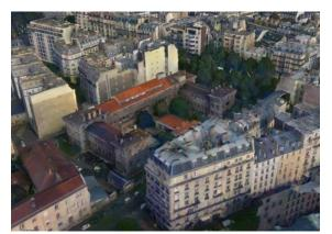
The new 3D Mesh Layer (3DML) technology supported by TerraExplorer allows users to load and query fully textured urban models that have been compressed and stream-optimized to accelerate loading speed and efficiently handle memory. 3DMLs are created in TerraBuilder CityBuilder by merging 3D mesh models generated by TerraBuilder PhotoMesh and/or layers with individually referenced 3D models.
